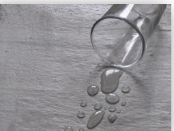
The treated surface achieves "Touch Dry" within 2 to 4 hours. Its water repellent properties progressively develop within 24 hours. Attainment of maximum properties in 5 days.
